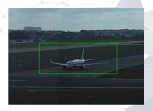
The system allows you to select or search for a target, using machine learning techniques, and follow it with the PTZ camera.
